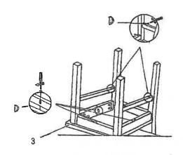
There are no pre-drilled holes to attach the seat
